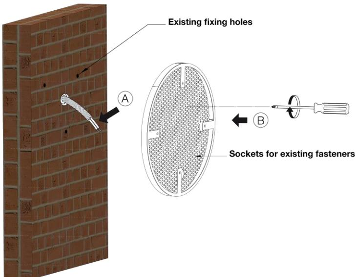
Insert the power supply cable through one of the two ø27 cable entries.
