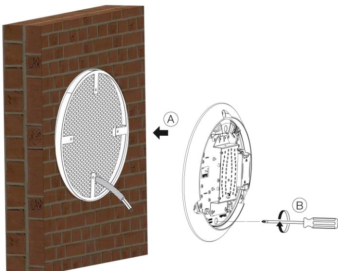
Fix the luminaire (VOILA or EFFICE) to the bracket using the fixing kit supplied.
